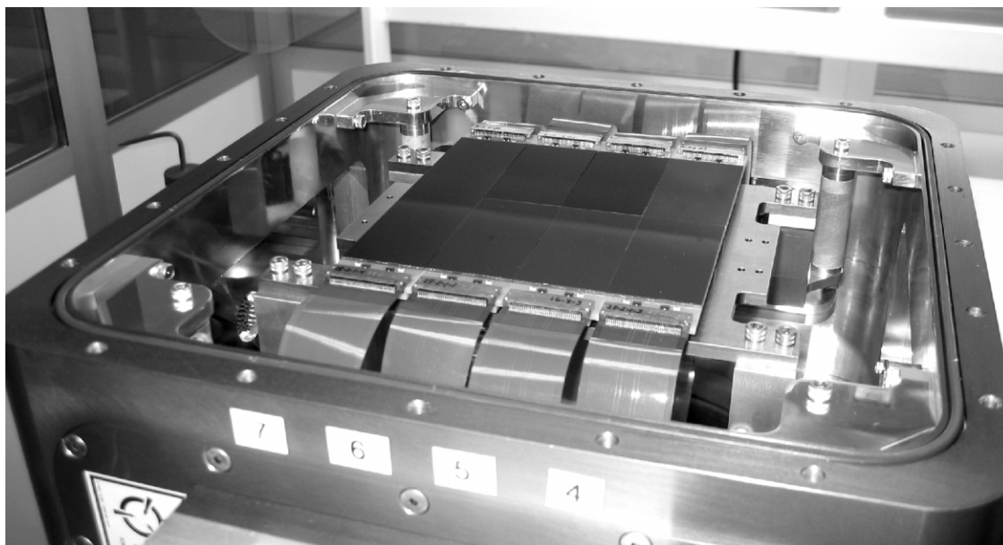
FIG. 8.—UHWFI 8K CCD focal plane populated with CCID-20 deep-depletion CCDs.
