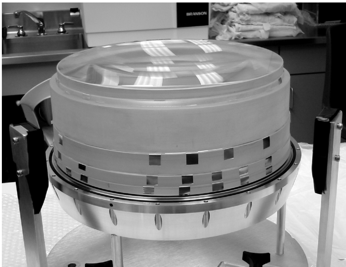
FIG. 6.—Lenses of the six-lens group, stacked with the front lens facing down on the lens cell front ring.
