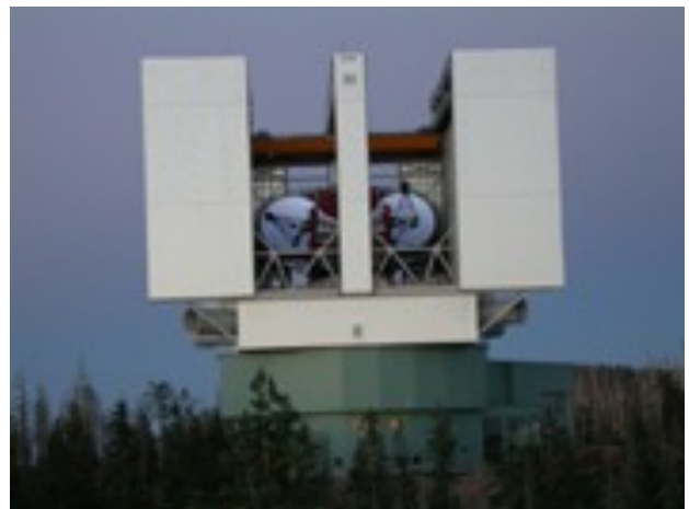
Figure 9. The Large Binocular Telescope atop Mt. Graham in Arizona. Each of the two primary mirrors is 8.4 m in diameter and the telescope is being equipped with adaptive secondary mirrors.
